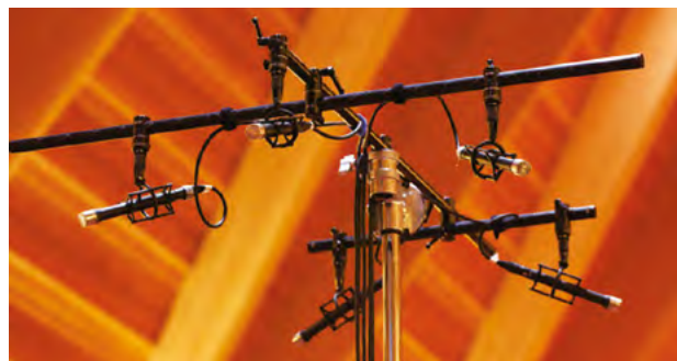
Figure 1 - Surround microphone configuration based on Decca Tree
